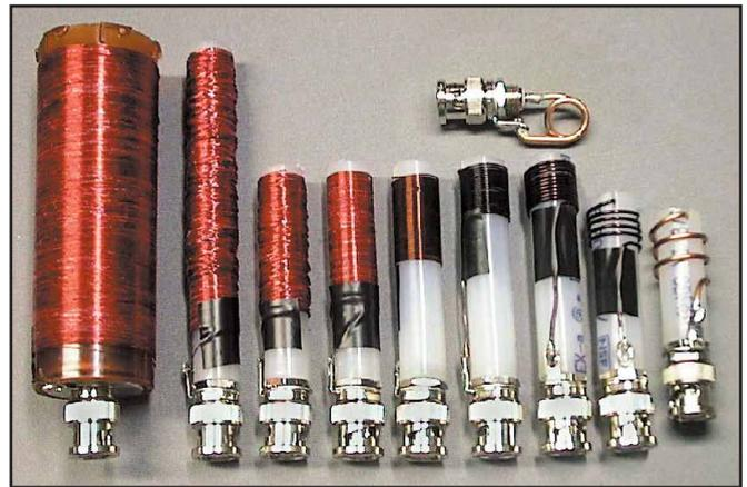
Figure 3—This is how the coils looked before the heat-shrink tubing was applied. Small pieces of electrical tape hold the turns in place during construction.
